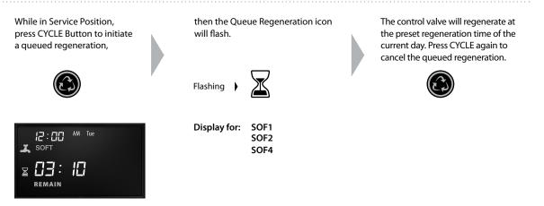
For SOF3, the display will alternate between **REMAINING GALLONS CAPACITY** and **REGENERATION TIME**. The valve will start to regenerate when either **REMAINING GALLONS CAPACITY** = 0 or preset **REGENERATION TIME** reaches first.
